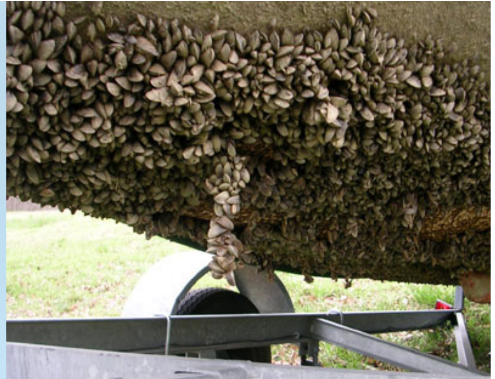
Heavy ZM buildup on hull greatly increases drag
