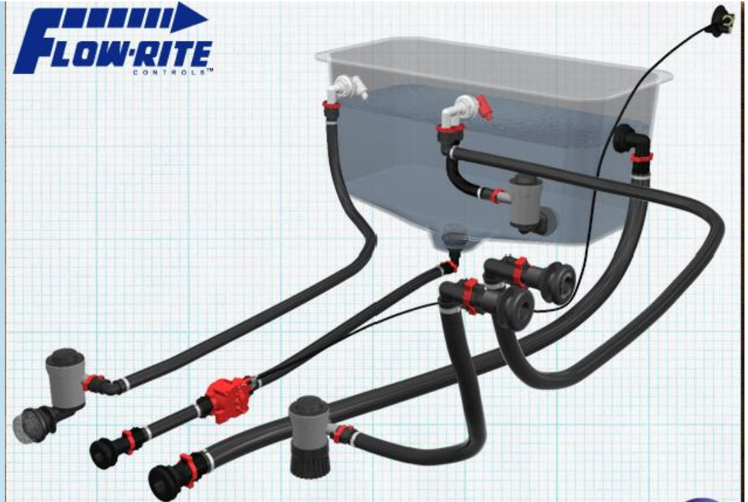
This live-well diagram illustrates the complex plumbing systems found in many fishing boats
